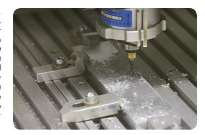
Reaming is difficult, and tool life is very low compared to that obtained in machining heat-treated, low-alloy steel.
